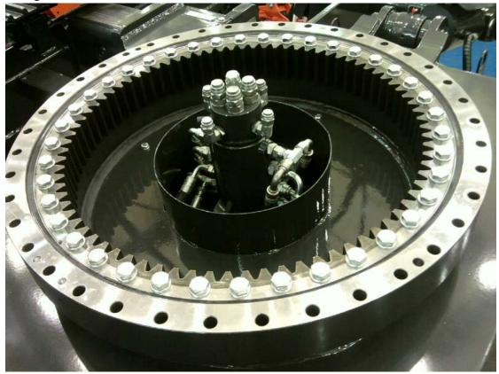
The excavator slewing ring is a kind of base parts of excavator. The quality of Slewing bearing directly affects the quality of construction machinery. The selection of the slewing bearing is the key affection to the design and performance of mainframe structure.
