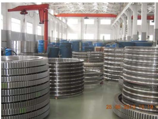
Lida has two production lines. One is for small and middle slewing ring bearings with the diameter less than 2.5 m and the other one is for big and heavy slewing ring bearings with the diameters between 2.5 m and 6 m. With our gear hobbing machine, we are able to make gears with 50 modules and
